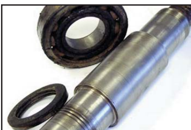
Shaft damage from a Labyrinth Seal.
