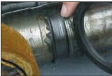
Shaft damage from Lip Seals.
